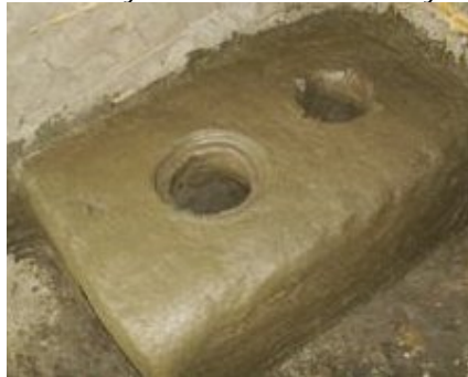
Photo 1: Energy saving stove built by a farmer beneficiary to conserve the environment
